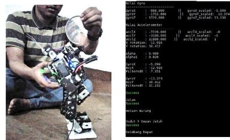
Gambar 5 Pengujian Output Tilt Angle Y Tanpa Filter
